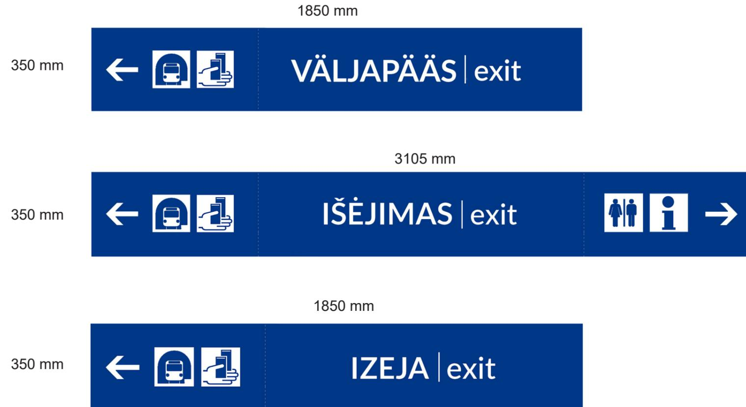
Typical dimensions of a single-line sign
